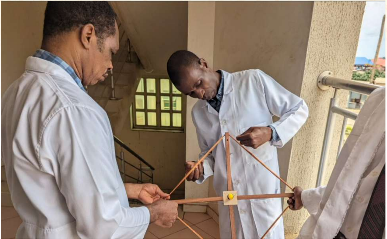
The research team, winding the aerial of the VLF Antenna at the AUL Space Lab.
