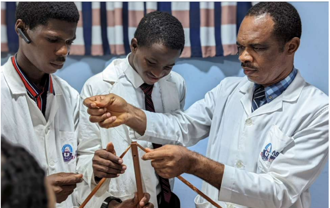
Dr. Victor U. J. Nwankwo with the research team, winding the aerial during the installation of the VLF Antenna at the AUL Space Lab in May, 2022.
