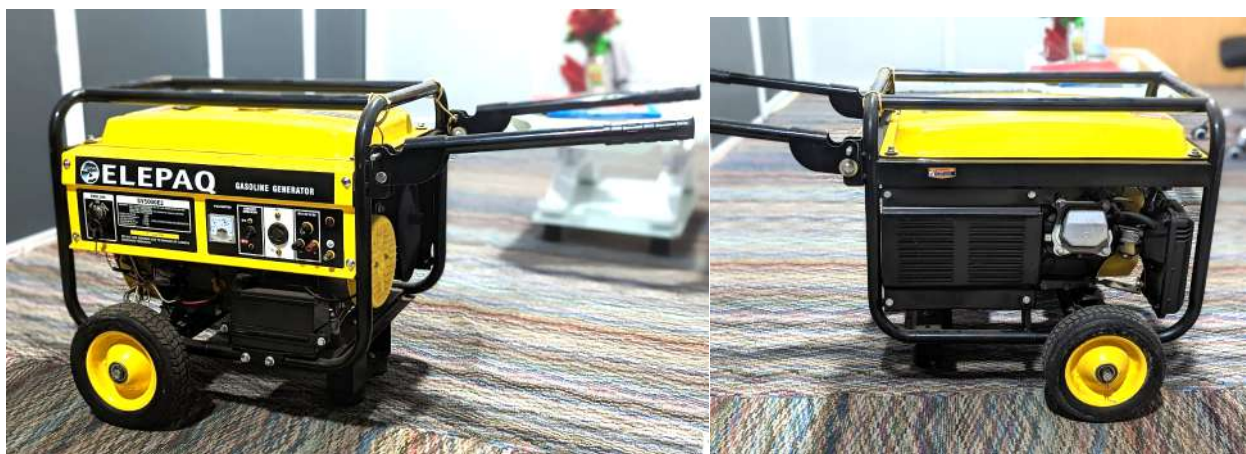
4.5 KVA electric power generating set for the AUL Space Lab
